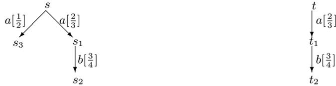
**Fig. 1.** Fuzzy bisimilarity is strictly finer than fuzzy simulation equivalence
